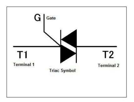
The TRIAC is a three-terminal device similar in construction and operation to the SCR. The TRIAC controls and conducts current flow during both alternations of an ac cycle, instead of only one. Both the SCR and the TRIAC have a gate lead. However, in the TRIAC the lead on the same side as the gate is "main terminal 1-MT1, T1 or even A1," and the lead opposite the gate is "main terminal 2-MT2, T2 or even A2."
